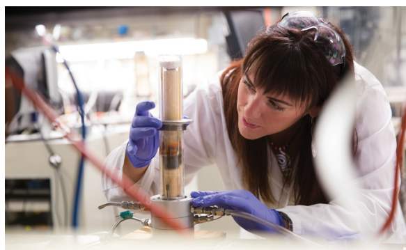
Top: The high temperature electrolyzer converts CO 2 into carbon monoxide, hydrogen, oxygen or syngas.
